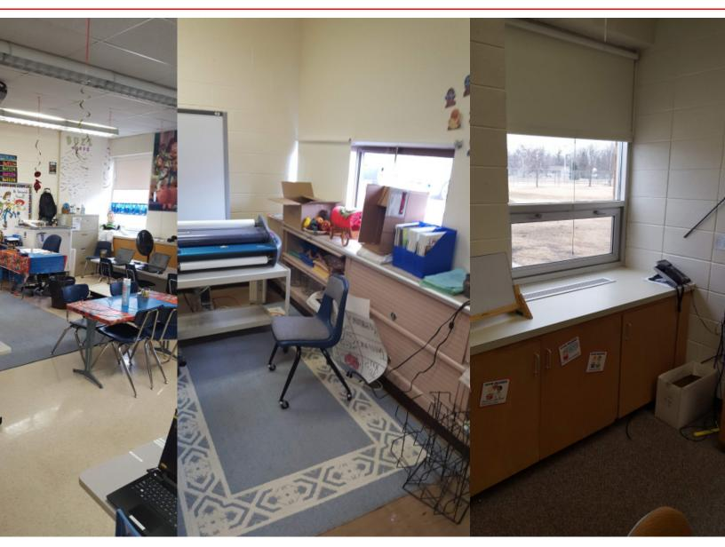
Corrective Action: Opening up the classrooms to more daylight by increasing the window area is recommended with window replacement. Daylighting and adequate area lighting has been shown to increase student achievement.
