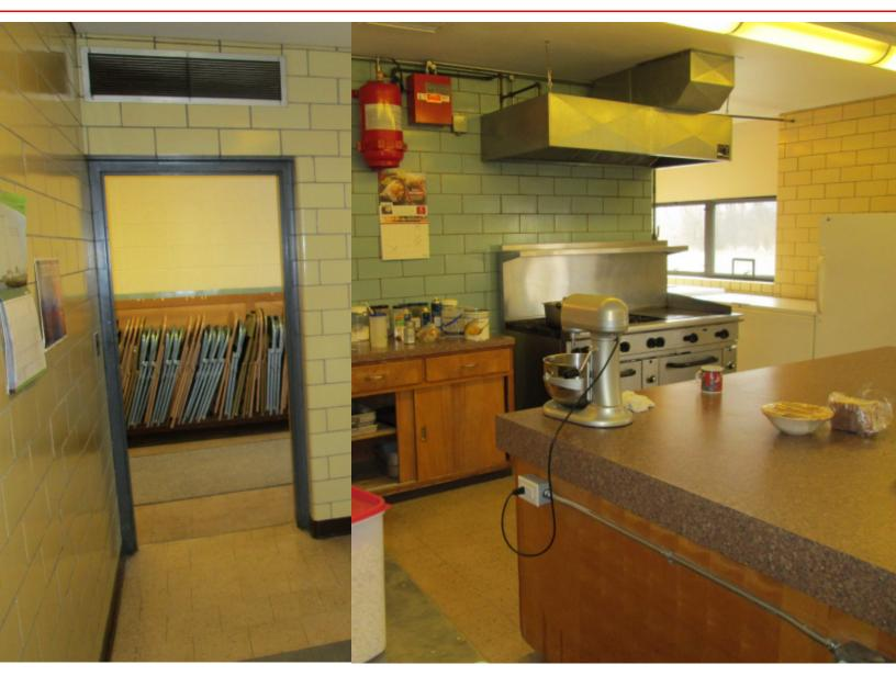
Corrective Action: Existing kitchen ventilation system does not meet current codes and would need to be replaced. Makeup air unit would need to be installed.
